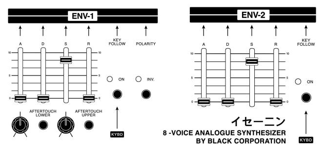
ISE-NIN features two envelope generators that are used to shape the sound over time. These envelope generators are typically labeled as Envelope 1 (ENV-1) and Envelope 2 (ENV-2).
