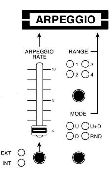
ISE-NIN's arpeggiator section allows for automatically playing and shifting notes harmonically in real time. This can be useful for improvising during a performance or for inspiring ideas while composing.
