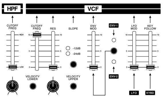
The filter section on the ISE-NIN synthesizer is an important component that can help shape the sound of your patches. It allows you to control the frequencies that are passed through the synthesizer, giving you the ability to create more complex and interesting timbres.
