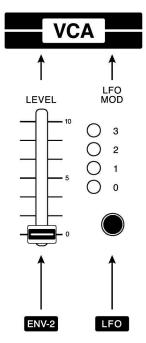
VCA section is responsible for controlling the volume or amplitude of the sound signal that passes through it. In the ISE-NIN, this section will likely include controls for adjusting the level of the audio signal, as well as controls for shaping the envelope that controls the VCA.
