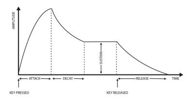
ENV-1 and ENV-2 have different routing options. In the ISE-NIN synthesizer, ENV-1 can be routed to control parameters, such as filter cutoff, oscillator pitch, or pulse width modulation, while ENV-2 is typically used to control the amplitude of the sound and filter.
