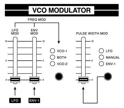
This section sets the amounts which the various modulation sources are applied to the pitch of VCOs 1 and 2: This section also controls modulator amounts to vary the width of PULSE when selected in either or both VCOs.
